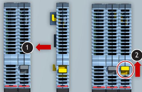
The positive "click-to-lock" mechanism firmly clamps Flexslice modules to each other to form a Flexslice station. Simply push each module together and slide the quick release locks into position.
