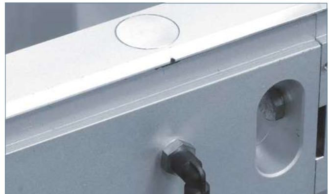
Lubrication point in guide rail
