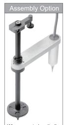
When mounted vertically, the Screw Rail can be used to simultaneously lift and rotate (Z-theta motion). With one motor driving the screw and a second rotating the rail, a compact, self-supporting pick and place mechanism can be created.
