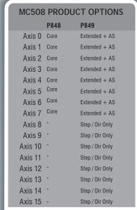
CORE AXES – can be configured in software as pulse and direction outputs to stepper or servo drives. They can also be configured for incremental encoder feedback or simulated encoder output
