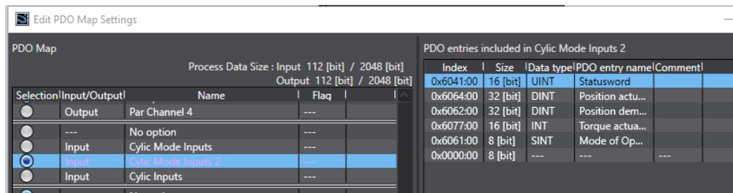
3. For cyclic PDO transmission of any drive value/parameter choose **Par Channel X** for Output and **Mon Channel X** for Input.
