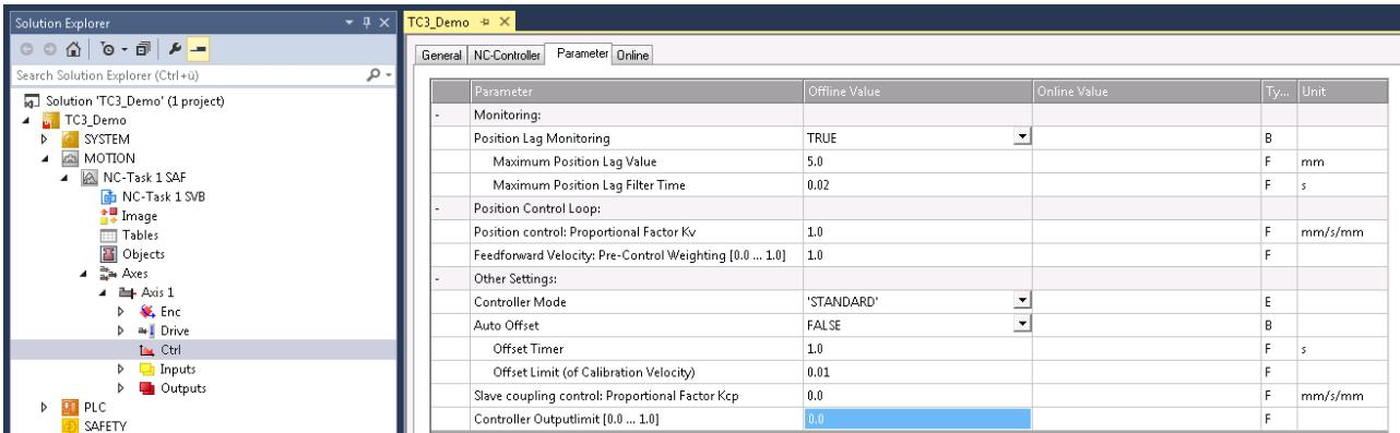
Though the position controlling is done in the drive the controller output has to be set to 0. If this is forgotten, the behaviour could be noisy. To set these NC parameters they have to be downloaded.
