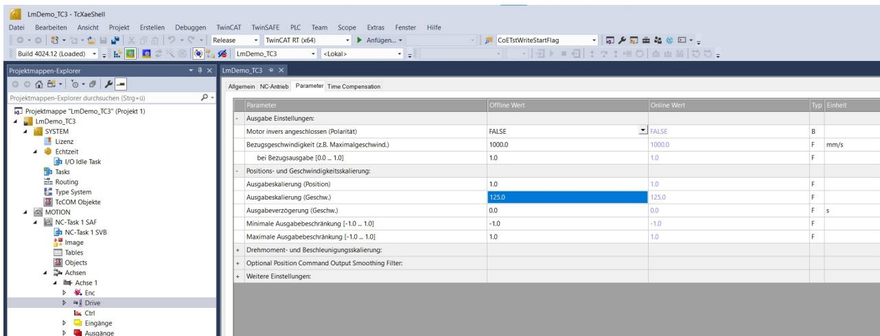
Then the velocity output scale factor has to be set to 125.0 for correct operation
