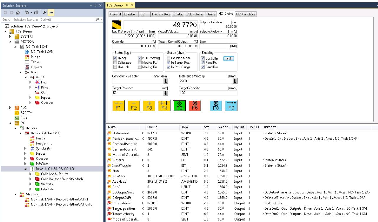
Now the servo drive can be used with system manager NC functionality when started.
