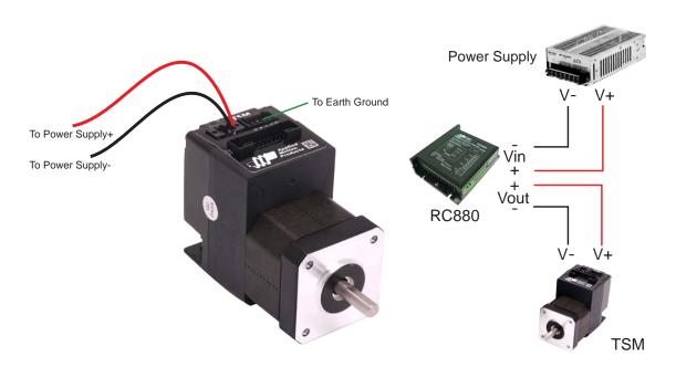
Applied Motion Products offers two matched power supplies for use with the TSM. A 24VDC, 150W(P/N PS150A24) and a 48VDC 320W(P/N PS320A48). These power supplies have current over load capability making them ideal for use. (To use with a switch power supplier, a RC880 regen must be connected in system)
