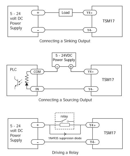
Do not connect the output to more than 30 volts. The current through the output terminal must not exceed 100mA.
