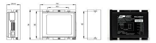
When using a regulated power supply you may encounter a problem with regeneration. The kinetic energy caused by regeneration is transferred back to the power supply. This can trip the overvoltage protection of a switching power supply, causing it to shut down.
