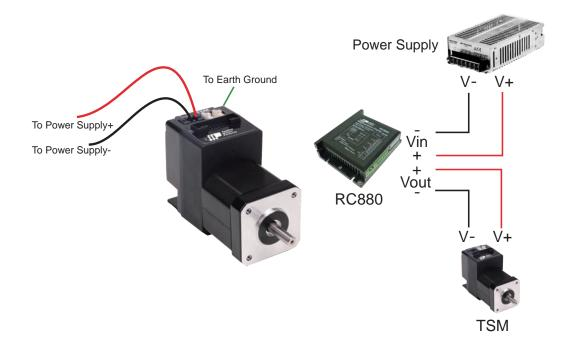
Applied Motion Products offers two matched power supplies for use with the TSM17C. A 24VDC, 150W(P/N PS150A24) and a 48VDC 320W(P/N PS320A48). These power supplies have current over load capability making them ideal for use. (To use with a switch power supplier, a RC880 regen must be connected in system)
