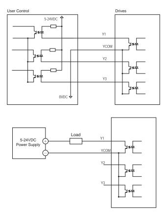
Do not connect the output to more than 30 volts. The current through the output terminal must not exceed 100mA.
