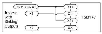
Connecting to Indexer with Sinking Outputs
