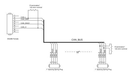
R termination: Network must be terminated at each end with a 120 ohm resistor.
