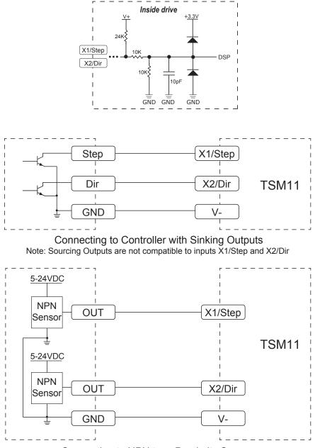
Connecting to NPN type Proximity Sensor Note: PNP type Proximity Sensor is not compatible to inputs X1/Step and X2/Dir
