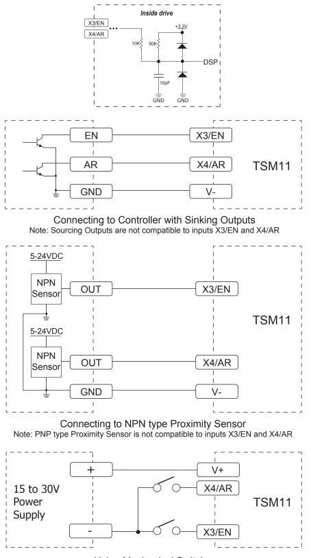
Using Mechanical Switches
