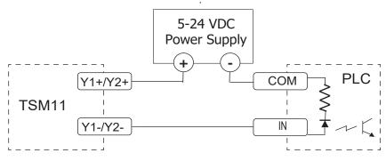
Connecting a Sourcing output with PLC's input
