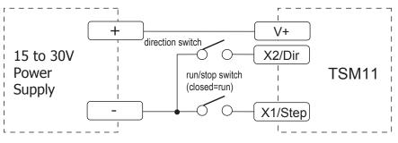
Using Mechanical Switches
