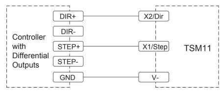
Connecting to Controller with Differential Outputs
