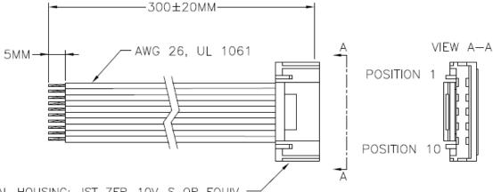
TERMINAL HOUSING: JST ZER-10V-S OR EQUIV. - CRIMP JST SZE-002T-P0.3 OR EQUIV. (10X)
