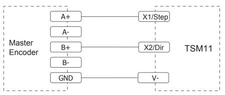
Wiring for Encoder Following with Differential Outputs
