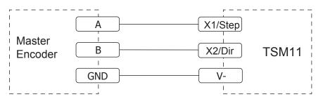
Wiring for Encoder Following with Single-ended Sinking Outputs
