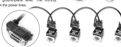
NOTE: Due to gauge of the main power lines, it is not recommended to use the "Add-A-Motor" cables with the larger 34 frame SmartMotor. If there is just one 34 frame SmartMotor in a system design, then it should be the first motor in the chain so as to minimize voltage drop effects over the entire network.
