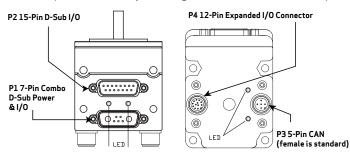
CAUTION: Pins 14 and 15 are intended for use with DE series motors for control power only. Attempting to power a non-DE motor through those pins, as main servo-drive power, may result in immediate damage to the electronics, which will void the warranty.
