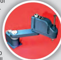
The Trio implementation of the SCARA robot allows from 2 axes to a full 6 axes with a 3 degrees of freedom wrist. There are also options to compensate for mechanical parasitic motion as well as different motor configurations.
